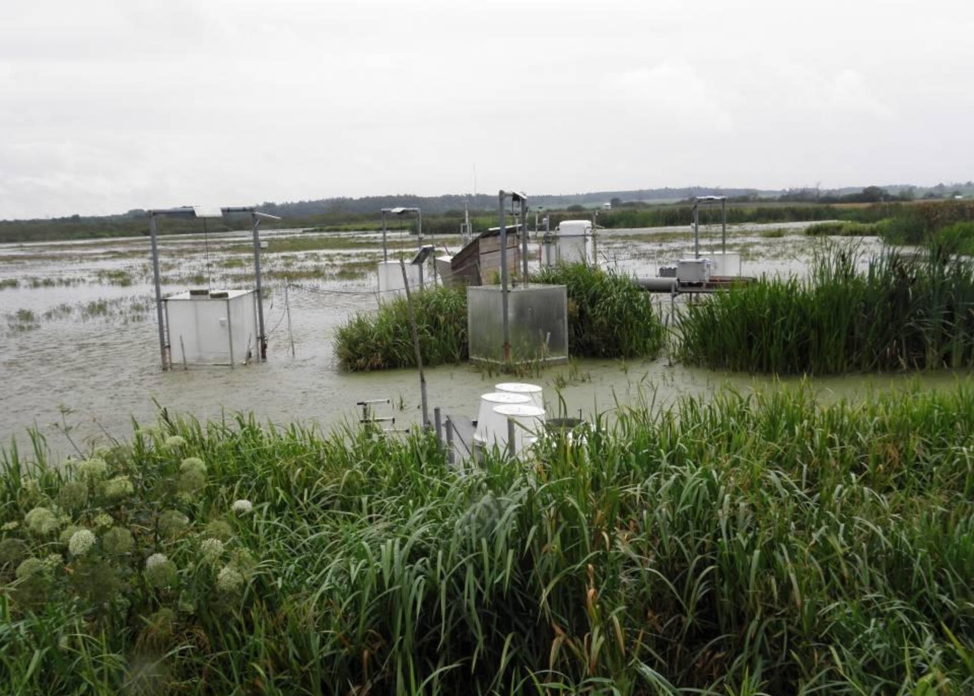
Messtation klimarelevanter Gase, Peenetal/Upost (MV August 2009) (Foto: M. Succow)
